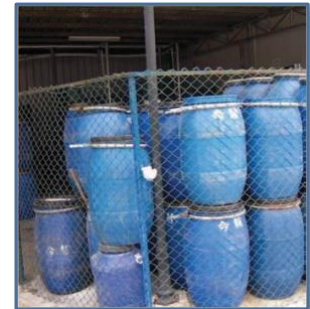
Good practice: Empty barrels stored in sheltered area reduces risk of stormwater pollution.
