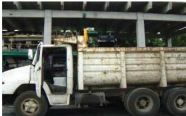
IA Bad Practice: This truck is not watertight and lacks the proper signage. It is unacceptable for bio-solid transport. Plastic lining is required to make watertight.
