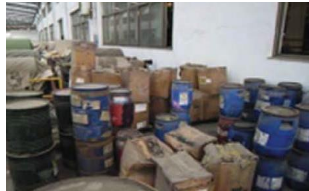
IA Incompatible wastes stored in a common area must have separate secondary containment structures to prevent mixing of incompatible waste streams.
