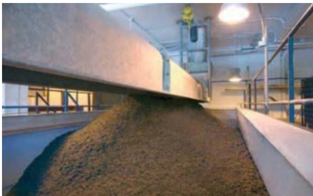
Good practice: Bio-solids ready for transportation after proper bio- solids management processing (i.e., thickened, stabilized, conditioned, disinfected, and dewatered).
