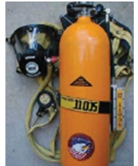
SCBA for emergency or planned entry into unknown concentrations or IDLH (Immediately Dangerous to Life or Health) conditions
